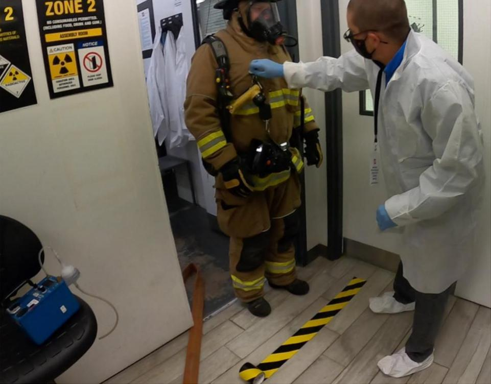
Photograph 30: MHPRA Taking a Swipe of a Boot Worn by the PFD
