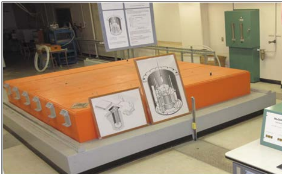
Figure 13-5: View of the top of the SLOWPOKE-2 reactor covered with concrete bricks
