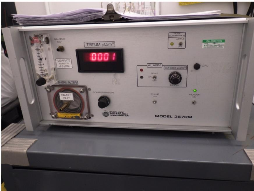
Figure 8. Fixed Tritium In Air Monitor Serial Number 2814
