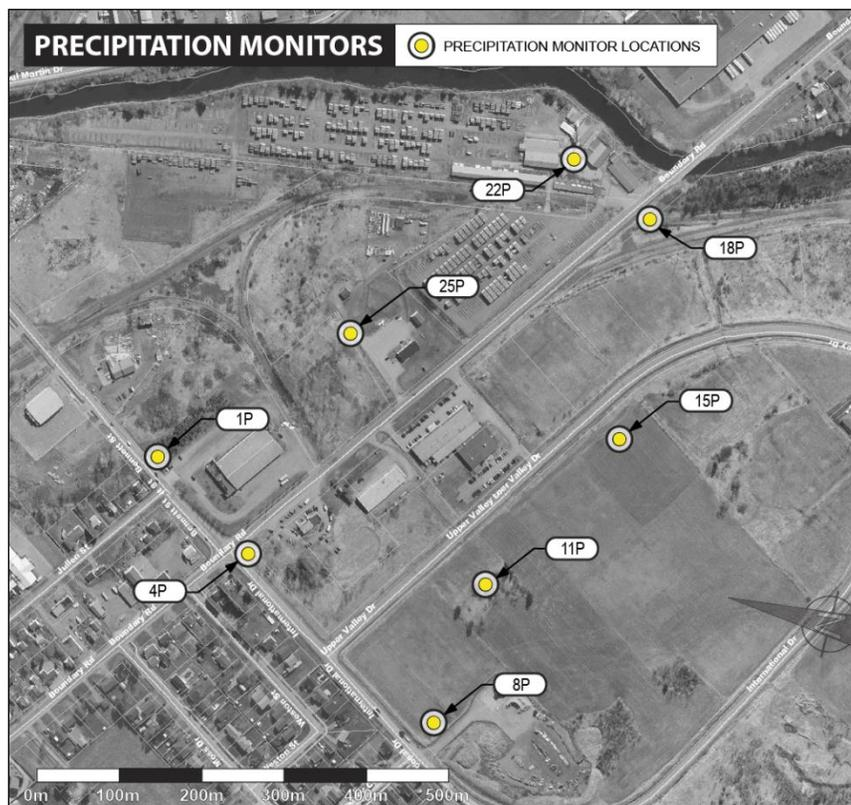
The samples were collected on a monthly basis by SRBT and a third party laboratory for tritium concentration assessment by the third party laboratory. Average results in 2016 ranged between 9 Bq/L (sampler 15P) and 43 Bq/L (sampler 18P).
