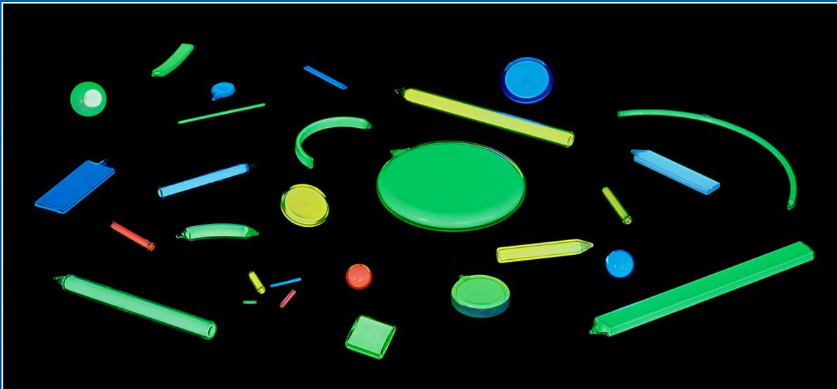
FIGURE B: VARIOUS TYPES OF TRITIUM LIGHT SOURCES PRODUCED BY SRB
