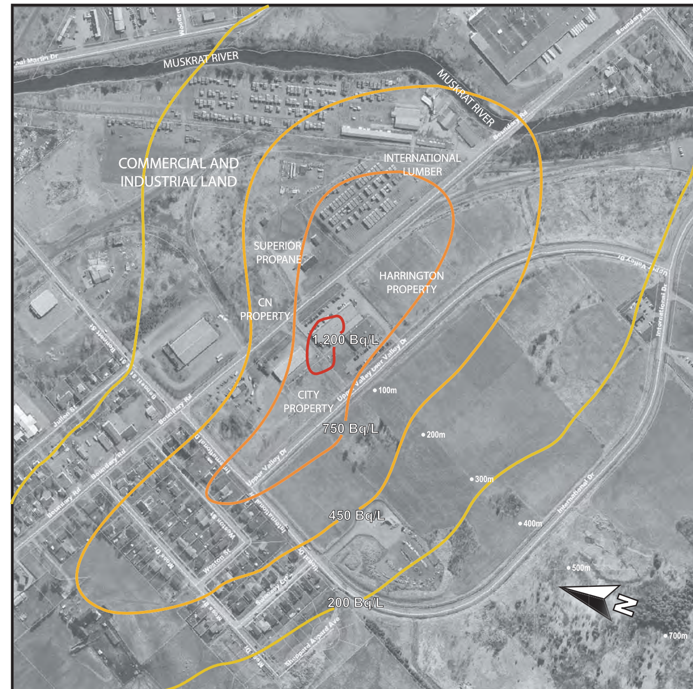
PREDICTED SOIL WATER CONCENTRATIONS BASED ON PROPOSED FUTURE EMISSION LIMIT OF 67 200 GBq/a
